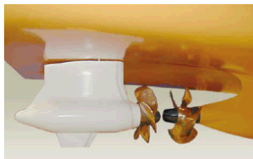
Modern contra rotating propellers
