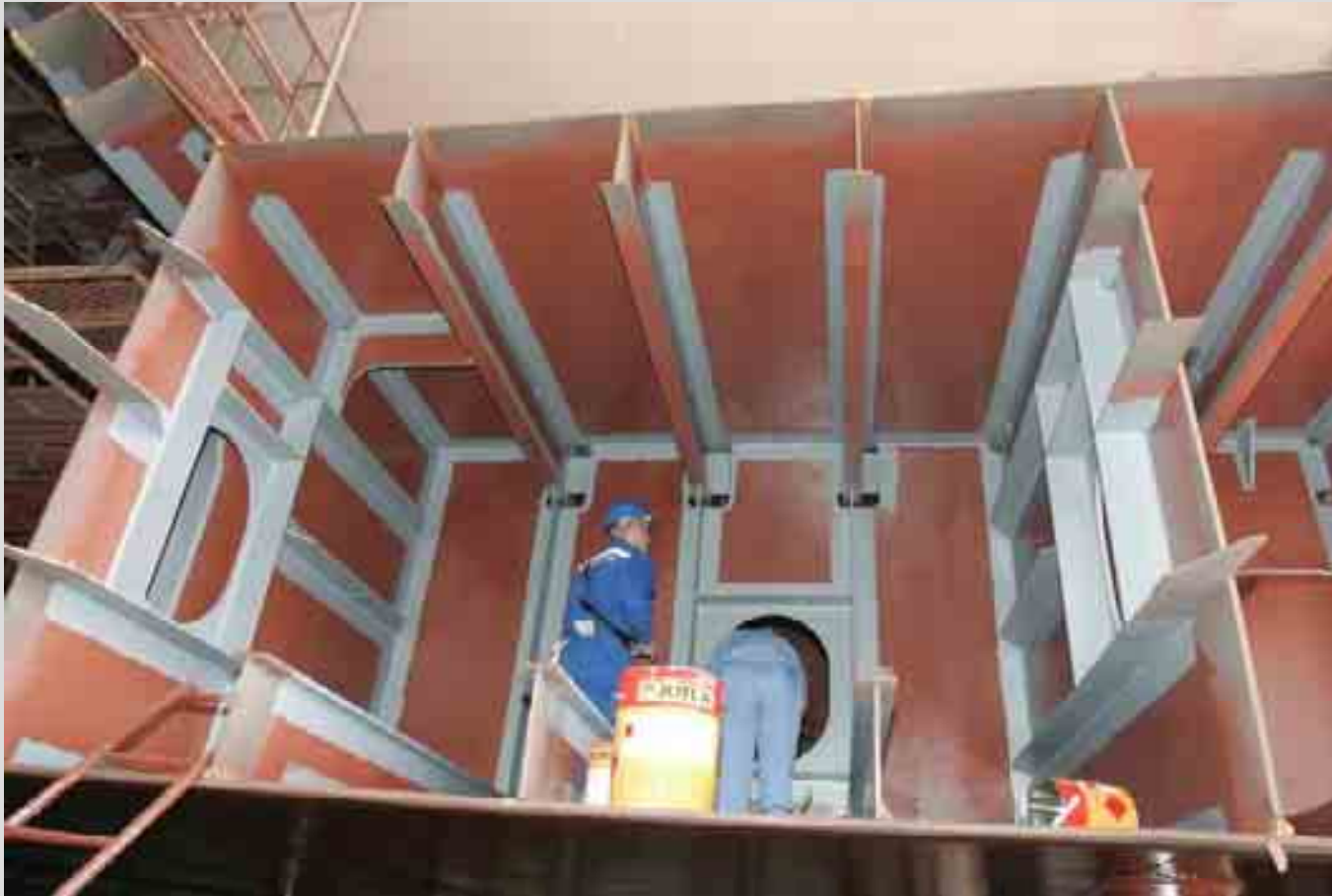
When it all goes well - high quality stripe coating and finishing
